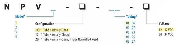
\*Use the chart below to identify the appropriate **Model** and **Tubing** based on the desired specifications.
