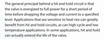
Clippard's hit and hold option minimizes the heat generated by the coil while dropping power consumption to 1/4, 1/9, or 1/16 of the rated power when the holding voltage PWM duty cycle is 50%, 33%, and 25% respectively. This option is available on Clippard NIV, PIV, and NPV series valves.
