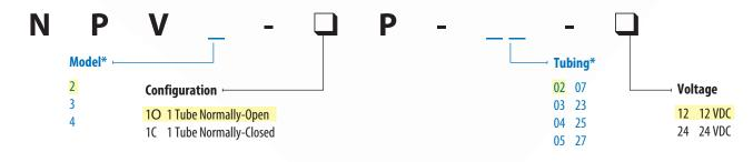
\*Use the chart below to identify the appropriate **Model** and **Tubing** based on the desired specifications.
